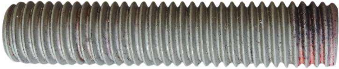
Figure: 3 Shows stud sample in DP tested condition. No significant indication is seen.
