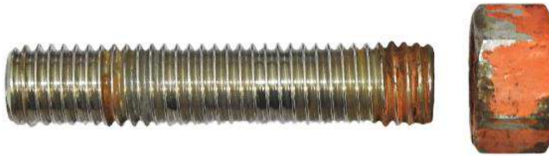
Figure: 2 Show sample after removing the nut. Brownish deposits are seen on the thread region. No significant damage is seen.
