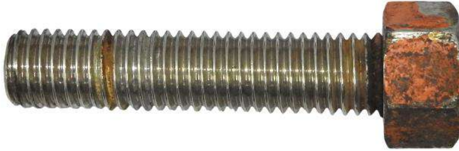
Figure: 1 Show stud sample in as-received condition. No significant damage is seen. Brownish deposits are seen on the nut and nearby thread region.
