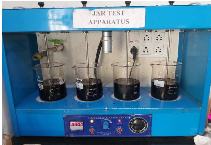
Figure 7.18: Onsite experimental setup of treatability studies
