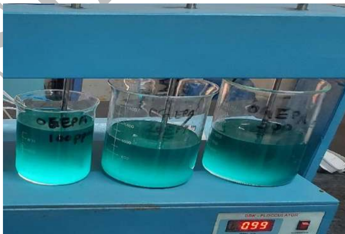
Figure 8.9: Picture showing Post Physico-chemical treatability studies for CETP OGEPA
