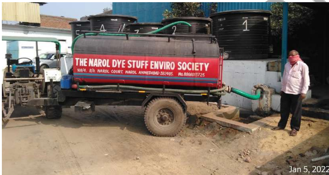
Figure 6.2: Raw effluent unloading through tankers at CETP Narol Dye Stuff
