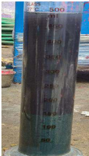
Figure 8.4: Aeration tank Biomass settling in 30 minutes
