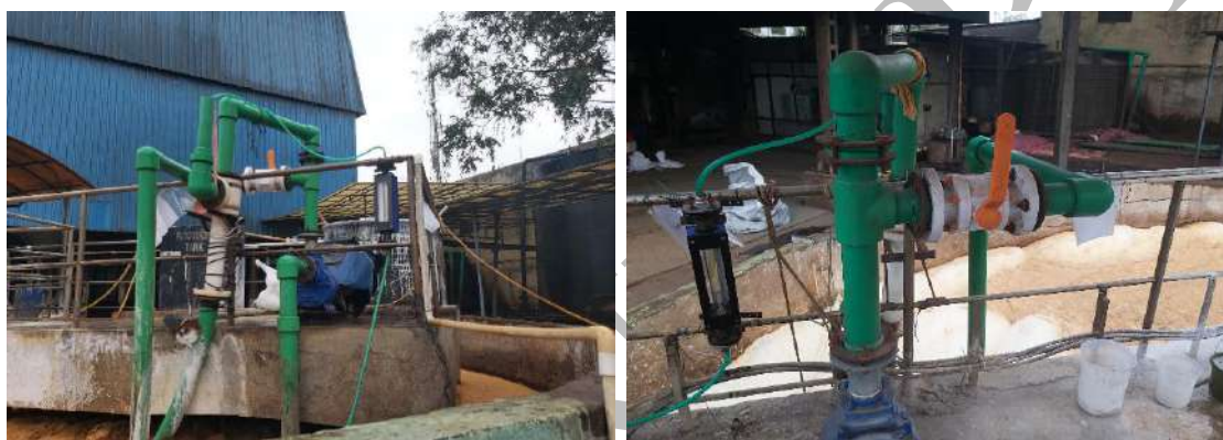
Figure 9.9: Picture showing trial runs of hydro-dynamic cavitation at CETP premises
