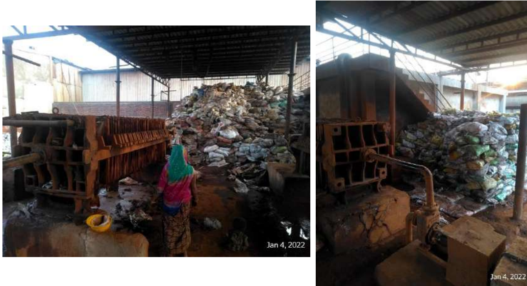
Figure 5.8: Picture showing storage of dewatered sludge
