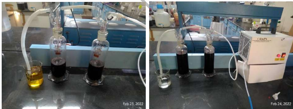
Figure 17.19: Bench scale experimental setup of ozonation based treatability studies
