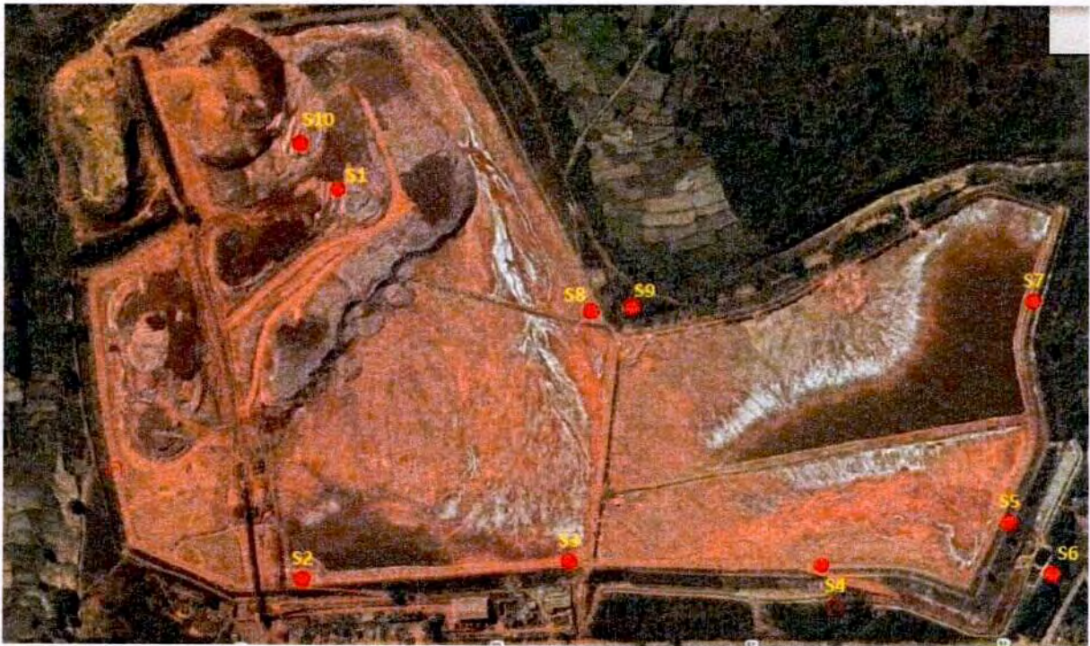
Fig. 3.2 An image showing locations of borelogs for soil investigation on the RMP
