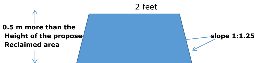
Cross- section of water body protection embankment
