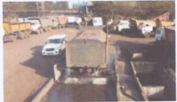
Mechanized wheel washing system
