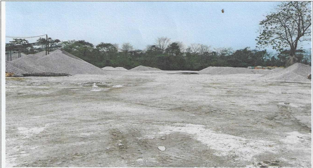
Picture: Time to time wetting of the premises of the stone crusher, so as to avoid fugitive emission.
