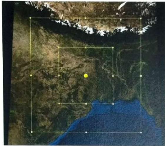
Figure 5.4: AERMOD grid covering the Jharia Coal Fields (JCF). The line, area, and point sources covered in the study are indicated in red color. The UTM coordinates of the left bottom point are x=406111 and y=2603492 , and the coordinates of the right top point are x=456248 and y=2653417 .
