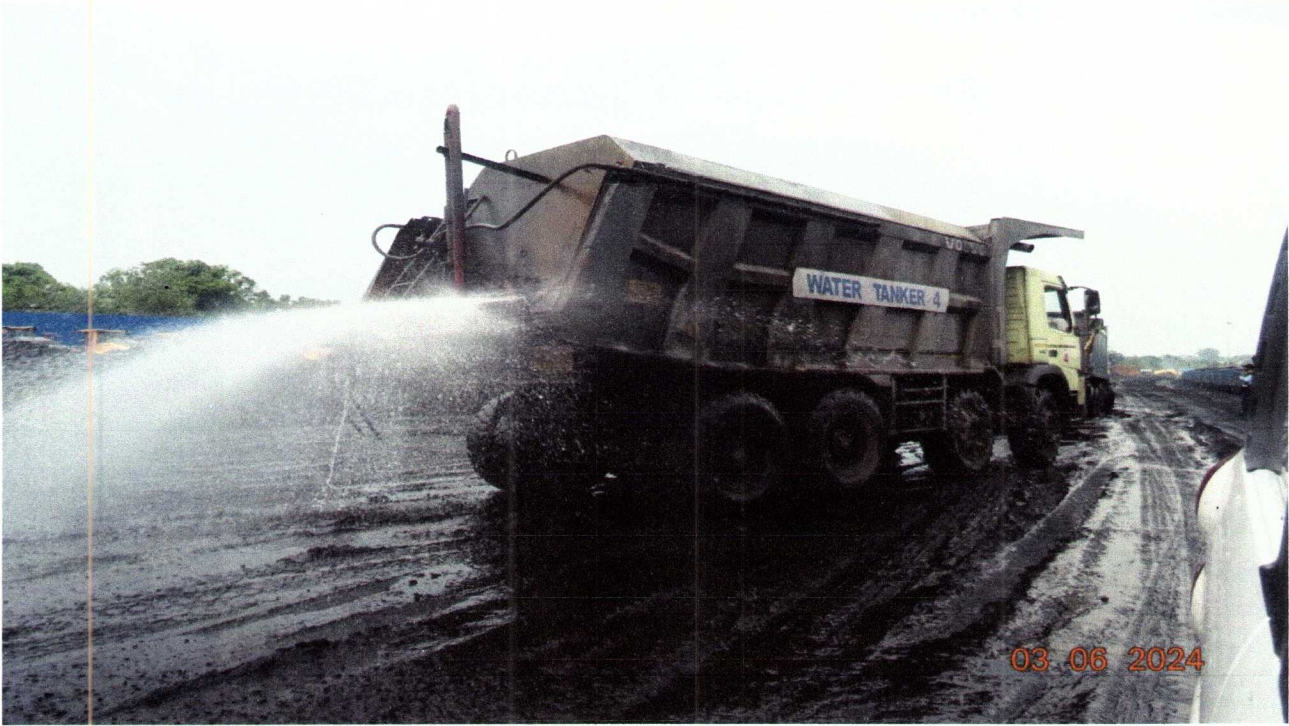
➤ Water sprinkling at Dumka Siding
