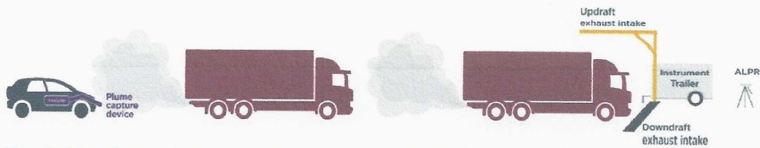
Figure 3a: Schematic setup of a plume chaser installed in vehicle measuring the exhaust emissions from the truck in front
