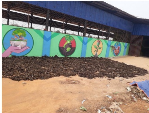
Figure 27: Compost put for drying for stabilization
