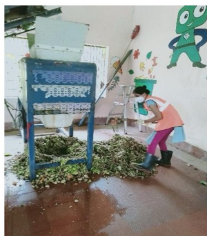
Figure 18: Collecting shredded waste to load in tubs
