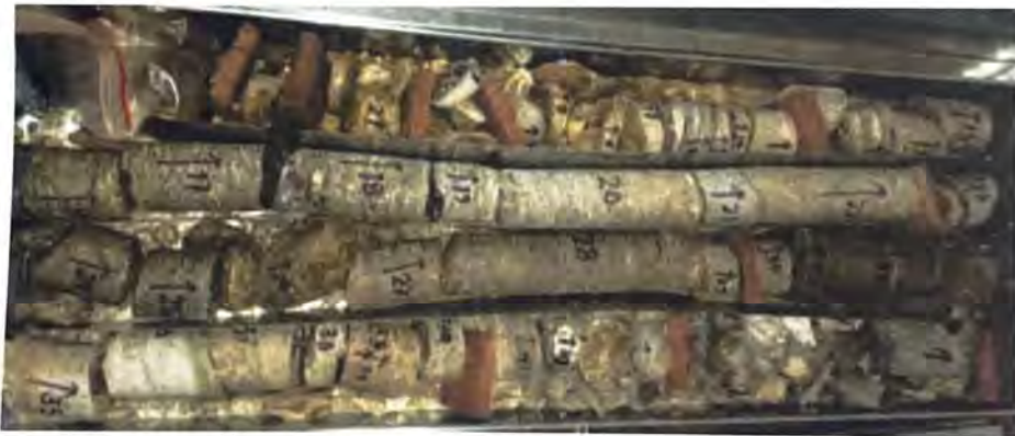
Photo 02:-core box showing recovered core samples from various depth of Bore hole no.02.
