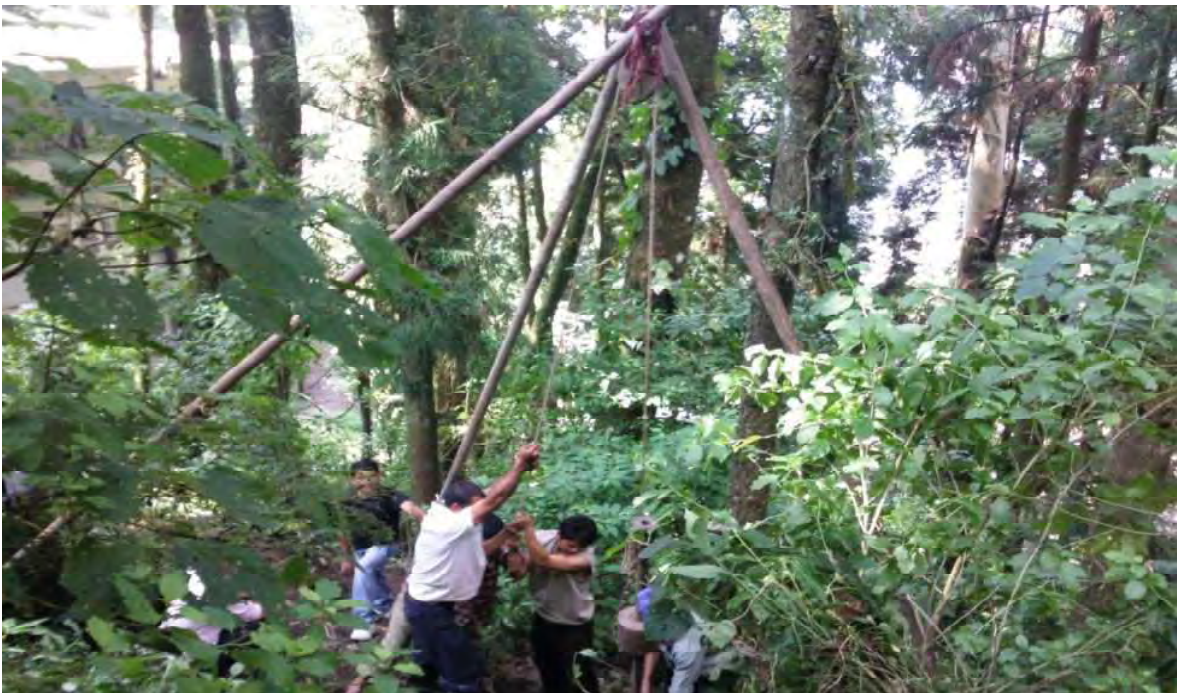
Soil Sampling on progress at Western slope of Tashiling Secretariat
