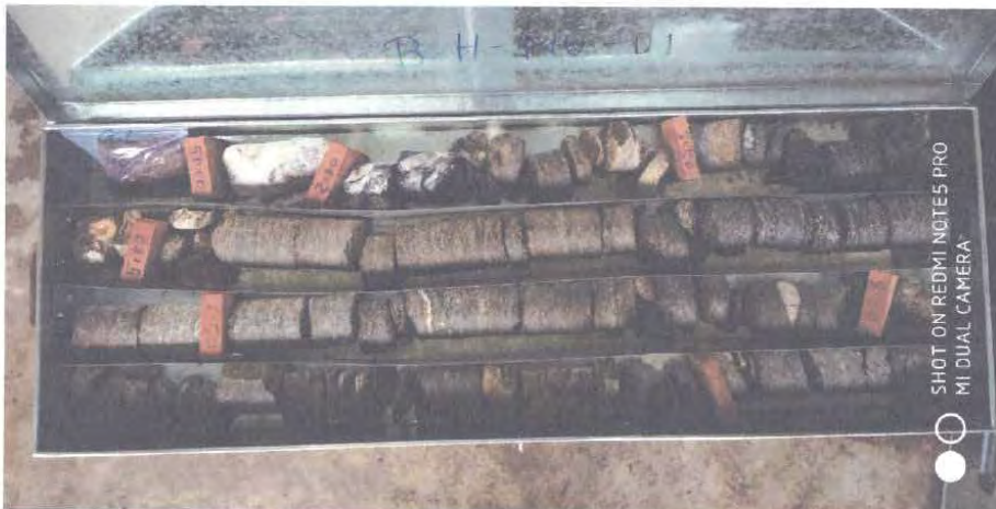
PHOTO;- CORE RECOVERY AT BH-01 LOCATION.
