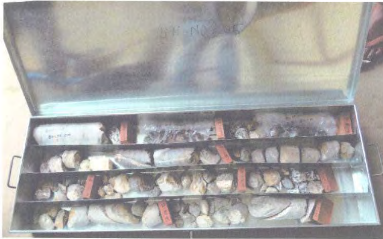
FIG;- CORE RECOVERY AT LOCATION BH-05.
