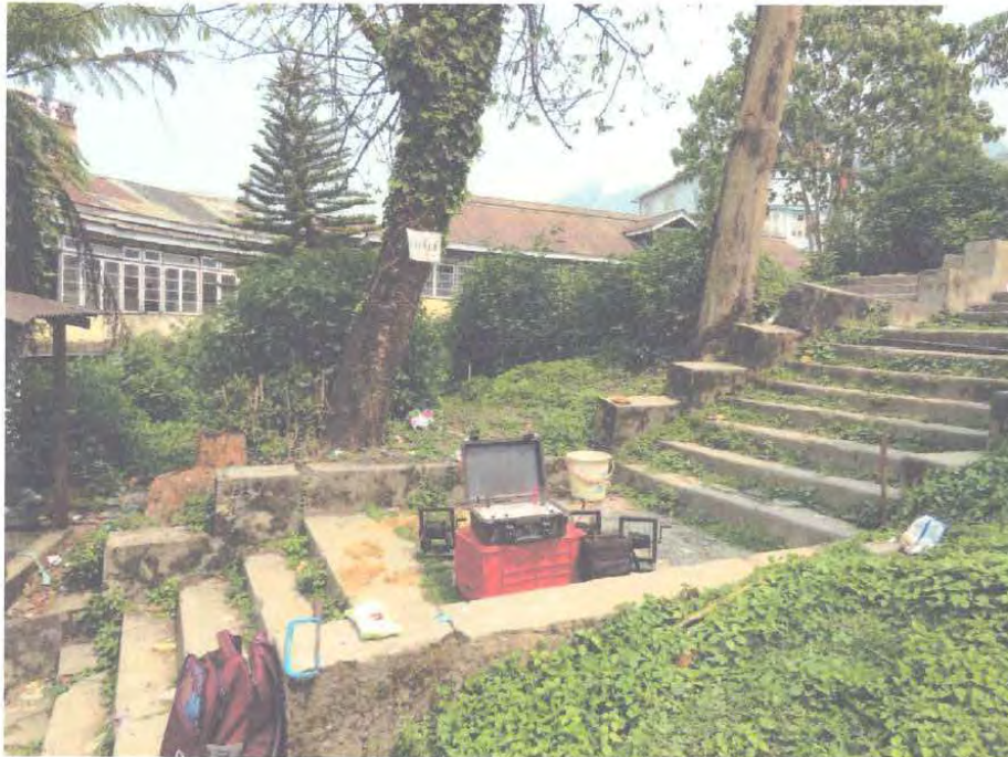
Photo:-Electrical resistivity Profiling Survey is at progress along, N20°W-S20°E direction at site.
