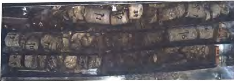
Photo 01:-core box showing recovered core samples from various depth of Bore hole no.01.
