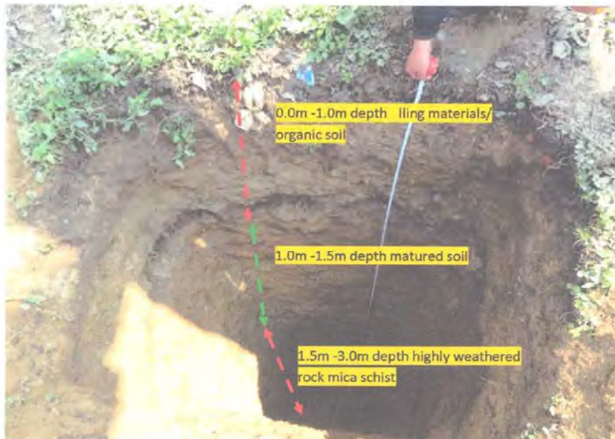
Fig;- Soil profile of the Pit-01 at old west point school complex, Gangtok.
