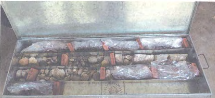
FIG;- CORE RECOVERY AT LOCATION BH-04.
