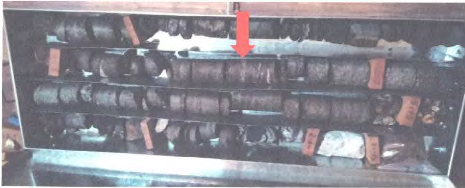
Photo 01: core box showing recovered core samples from various depth of Bore hole no.01.
