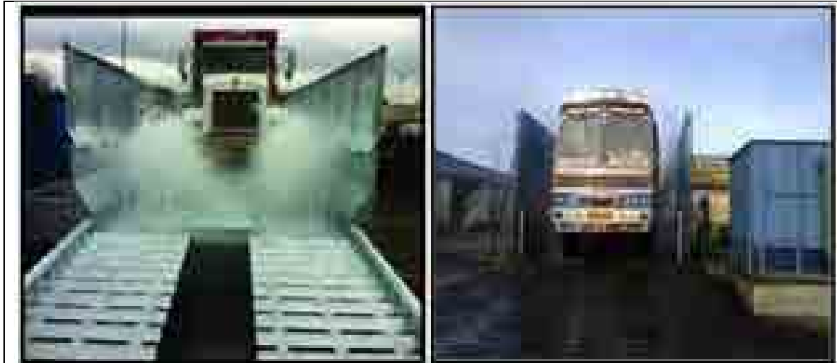
Exhibit 5-4: Automatic Tyre Wash System
