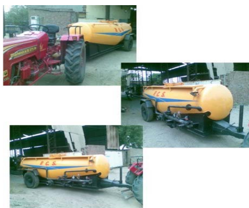
Small bulkers designed for transportation of flyash by tractors
